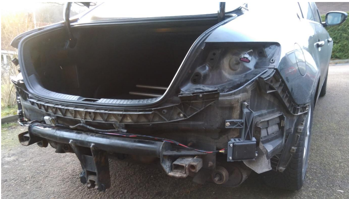
Figure 1 - Sensors, brackets and wire harness mounted behind bumper.
